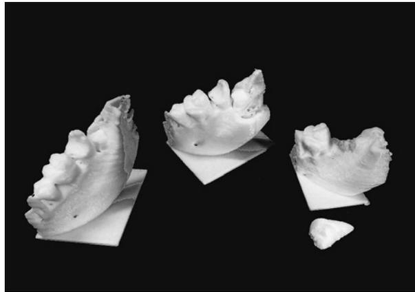
Fig. 2 Tooth-jawbone 3D models fabricated using 3D printer
