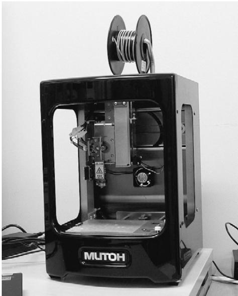
Fig. 5 Desktop 3D printer Value3D MagiX MF-500
